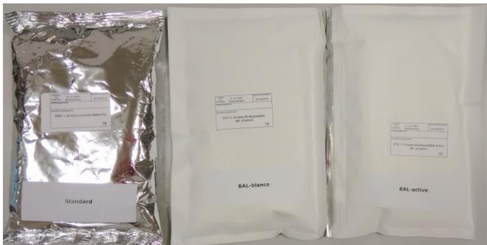
Figure 2. Comparison of the different packaging formats evaluated. Left: conventional packaging, middle: project developed structure (passive), and right: active packaging structure.
